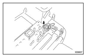
Disconnect the connector and remove the amplifier. (b)
