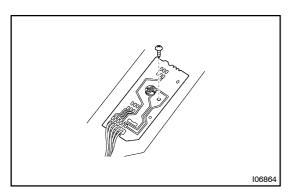
Remove the screw and switch. (b)
