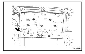
(b) Remove the 4 screws and heater control, then disconnect the connectors.
