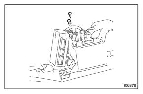
(c) w/ Rear Heater: Remove the 2 screws and amplifier.
