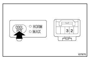
(b) Check the continuity exists between terminals 2 and 3 while switch is pressed.
