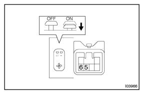
(c) Check the continuity exists between terminals 5 and 6 while switch is pressed.
