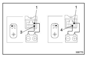
(b) Connect the positive (+) lead from the battery to terminal 1 and negative ( -) lead to each terminal, then check that the "LO" and "HI" indicators light up as shown in the chart.
