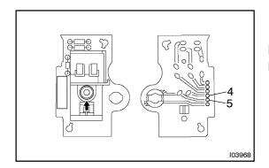
(2) Check the continuity exists between terminals 4 and 5 while switch is pressed.
