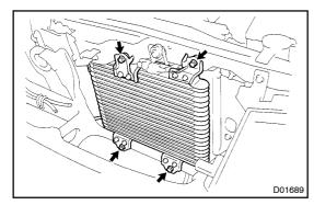
(b) Remove the 4 bolts and oil cooler.
