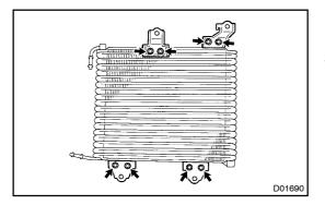
(c) Remove the 8 bolts, oil cooler bracket and stay.
