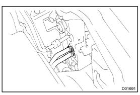
(a) Loosen the 2 clips and disconnect the 2 hoses.
