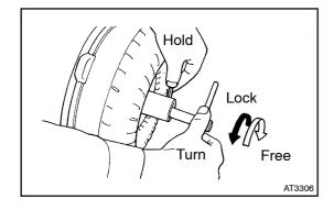
(c) With the torque converter standing on its side, the clutch locks when turned counterclockwise, and rotates freely and smoothly clockwise.
