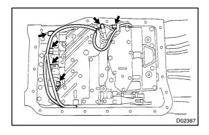
(e) Connect the 5 solenoid valve connectors and ATF temperature sensor connector.
