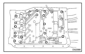
(b) Remove the 22 bolts and valve body.
