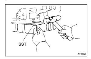
(b) Insert the blade off SST between the transmission and oil pan, cut off applied sealer, and remove the oil pan. SST 09032 -00100
