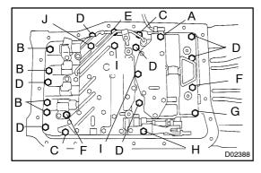
(b) Temporarily install the valve body with the 22 bolts.
