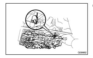
(c) Disconnect the throttle cable from the cam and remove the valve body.
