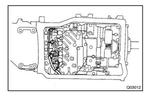
(f) Connect the 4 connectors to the solenoid valves.
