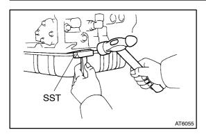
(b) Insert the blade off SST between the transmission and oil pan, cut off applied sealer, and remove the oil pan. SST 09032 -00100
