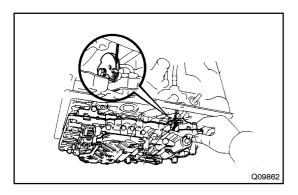
(b) Connect the throttle cable to the cam.
