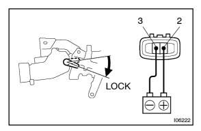
(b) Reverse the polarity and check that the door lock link moves to LOCK position.
