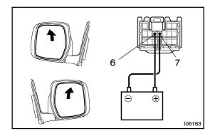
Connect the positive (+) lead from the battery to terminal (c) 6 and the negative (-) lead to terminal 7, and check that the mirror turns upward.
