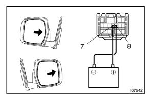
(b) Reverse the polarity, and check that the mirror turns to the right side.
