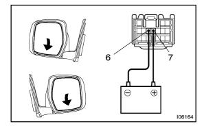
Reverse the polarity, and check that the mirror turns downward.
