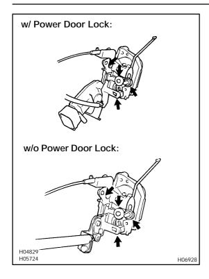
S Apply MP grease to the sliding and rotating parts of the door lock
