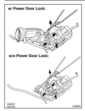
Apply MP grease to the sliding and rotating parts of the door lock.
