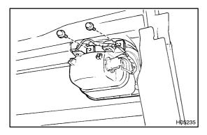
(b) Disconnect the connector, then remove the 2 bolts and high-mount stop light.
