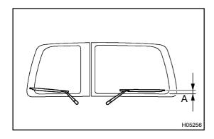
(d) Adjust the installation position of the wiper arm to the position shown the illustration.
