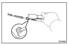
(c) Using a scraper, remove any excessive or protruding adhesive.
