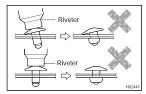
S Loose tightening may result from either tilting the riveter while handling or the riveter not connecting to the material.
