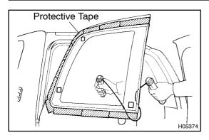
(d) Let the piano wire pass as shown in the illustration, cut off the adhered part to the clips.
