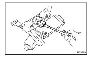
(c) Using a screwdriver, remove the cam plate cover.
