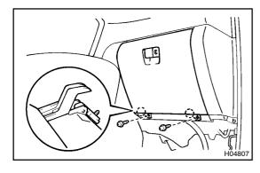
(b) Remove the 2 screws and glove compartment door as shown in the illustration.
