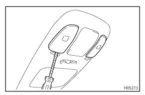
(c) Using a screwdriver, remove the 2 lenses.
