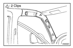
(b) Using a screwdriver , remove the front pillar garnishes. HINT:
