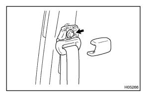
(b) Rear No.1 seat outer belt shoulder anchors Torque: 43 N·m (440 kgf·cm, 32 ft·lbf)
