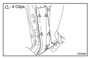
(b) Using a screwdriver, remove the center pillar lower garnishes as shown in the illustration.
