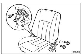
(d) Remove the 4 bolts and seatback assembly.
