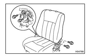
(c) Remove the 4 bolts and seatback assembly.
