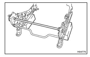
(c) Place the adjusters on a spacer to adjust the seat rail in parallel and install the connecting pipe.
