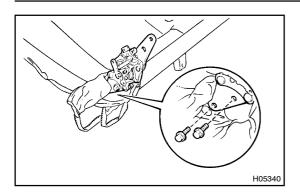
(c) Remove the 2 bolts and rear No.1 seat adjuster.
