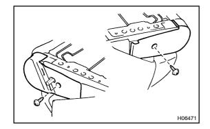
(c) Remove the 2 screws and 2 No.1 reclining covers as shown in the illustration.
