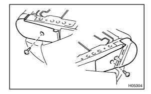
(c) Remove the 2 screws and 2 No.1 reclining covers as shown in the illustration.
