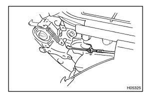
(b) Loosen the nut, remove the reclining connecting wire of LH side edge.
