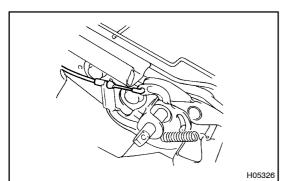
(c) Remove the reclining connecting wire of RH side edge.
