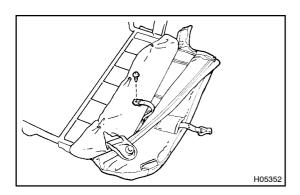
(c) Remove the screw, fold seat stopper band and seatback cover.
