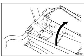
(b) Open the seatback cover, then remove the 2 hog rings as shown in the illustration.
