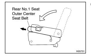
(d) When folding down the seat beck forward and extracting the seat belt slowly, check that the belt is locked after a certain length (approx. 500 mm (19.69 in.)) of the belt has been extracted.
