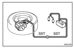
(2) Place the front seat outer belt on the ground and cover it with the disc wheel with tire.
