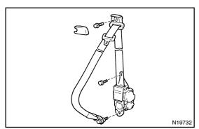
(c) Remove the 3 bolts and front seat outer belt.
