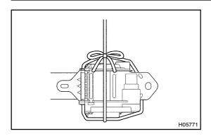
(c) As shown in the illustration, tie the seat belt pretensioner so that the vehicle front side of the pretensioner is facing downward and that the pretensioner is horizontal.
