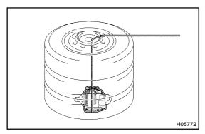
(e) Pile 2 tires and 1 tire with wheel around the seat belt pretensioner. Pass the cord through the wheel of the top tire.
