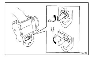
(d) Unlock the sensor by operating in the safety lock release lever as shown in the illustration.
