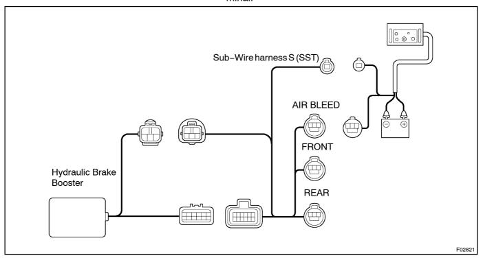
(d) Turn the ignition switch OFF, depress the brake pedal more than 40 times.
