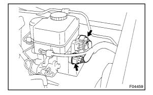
(a) Disconnect the 2 connectors from the hydraulic brake booster.
