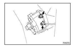
(c) Remove the 2 nuts and pump from the engine.
