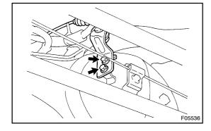
(c) Remove the 2 mounting bolts and shackle bracket.
