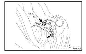
(c) Remove the speed sensor installation bolt and speed sensor from the steering knuckle.
