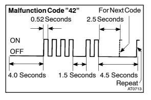
(2) The malfunction code is indicated, as shown in the chart on the left (DTC "42" is shown as an example).
