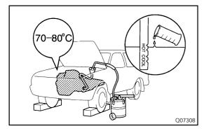
(3) With the engine OFF add new fluid through the oil filler pipe.
