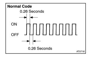
(4) Read the DTC indicated by the number of times the O/D OFF indicator light blinks.
