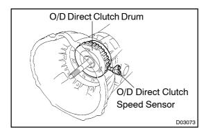
This sensor detects the rotation speed of the O/D input shaft from the rotation of the O/D direct clutch drum.
