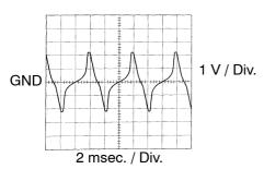
Refer to the chart for the wave form between terminals NCO and NCO  $\bar{}$  during engine idling.
