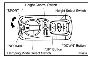
(b) Push the "DOWN" button of the height select switch 5 times or more within 5 seconds after starting the engine.
