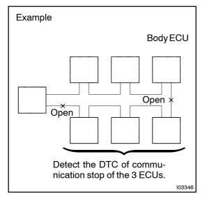
(c) If 2 communication buses are open at the position as shown in the illustration, DTC of ECU communication stop between those 2 buses is output.
