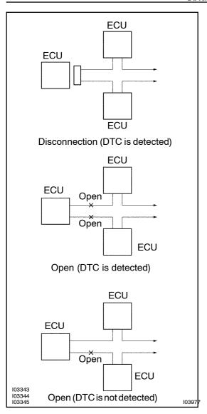
(b) If DTC of ECU communication stop is output, there is a possibility of connector disconnection or 2 communication buses open. It will not become abnormal with only communication bus open.
