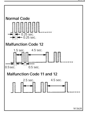
As an example, the blinking patterns for codes; normal, 12, and 11 and 12 are shown in the illustration.
