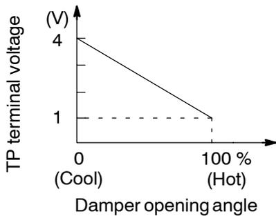
This sensor detects the position of the air mix damper and sends the appropriate signals to the A/C amplifier. The position sensor is built into the air mix damper control servomotor assembly.
