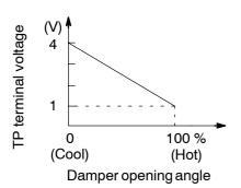
This sensor detects the position of the air mix damper and sends the appropriate signals to the rear A/C amplifier.
