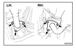
(b) Remove the 6 nuts and 2 gaskets from the exhaust man-
