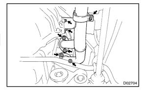
(b) Loosen the clamp bolt and disconnect the clamp from the support bracket.
