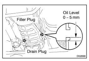
4. RAISE VEHICLE AND DRAIN TRANSMISSION OIL
