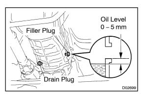
4. RAISE VEHICLE AND DRAIN TRANSMISSION OIL
