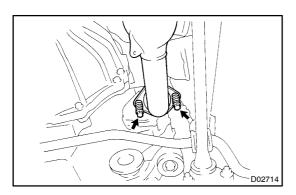
(b) Remove 2 bolts, springs and gasket from the exhaust manifold.
