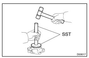
(b) Using SST and hammer, drive in a new oil seal. SST 09950-70010 (09951-07150), 09950-60010 (09951-00640)
