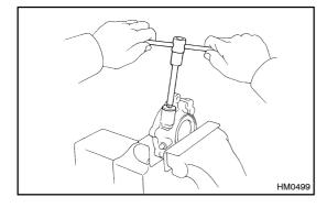
(f) Using a hexagon wrench, install and torque the screw plug.
