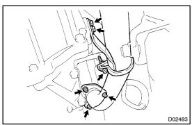
Loosen the clamp bolt and disconnect the clamp from the (b) support bracket.
