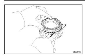
(d) Using a feeler gauge, measure the clearance between the synchronizer ring back and gear spline end.
