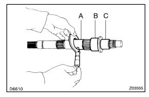
(b) Using a micrometer, measure the outer diameter of the output shaft journal.
