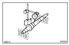
(c) Using a dial indicator, check the shaft runout.
