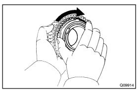
(c) Check the braking effect of the synchronizer ring. Turn the synchronizer ring in one direction while pushing it to the gear cone. Check that the ring locks.
