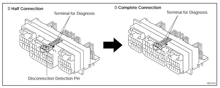
(4) Connector Twin–Lock Mechanism With this mechanism connectors (male and female connectors) are locked by two locking devices to increase connection reliability.
