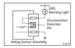
(3) Electrical Connection Check Mechanism
