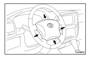
There should be no interference between the steering wheel pad and steering wheel, and the clearance should be uniform all the way around when the new steering wheel pad is installed on the steering wheel.
