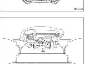
(1) Install the 2 bolts with washers in the 2 bolt holes in the steering wheel pad.
