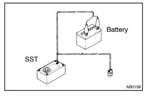
(1) Connect the SST to the battery.
