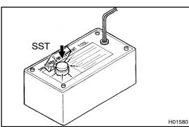
(2) Check functioning of the SST. Press the SST activation switch, and check that the LED of the SST activation switch lights up.
