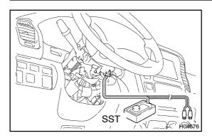
(3) Connect the SST connector to the airbag connector of the spiral cable.
