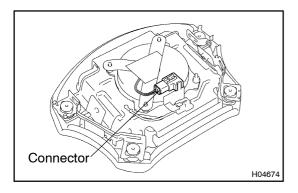
(b) Remove the connector on the rear surface of the steering wheel pad from the bracket.
