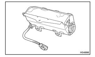
(a) Remove the front passenger airbag assembly.(See page RS-25)
