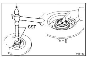
(b) Using SST, install a new oil seal into the hub. SST 09950-60020 (09951-00910),
