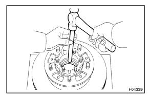
(b) Using a brass bar and hammer, remove the inside bearing outer race.
